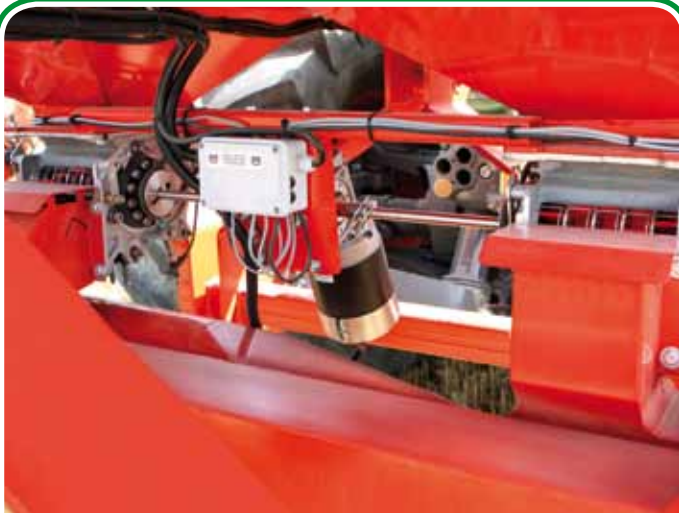
Distributori azionati dai motori elettrici gestiti dalla centralina GENIUS Distributors driven by electric motors that are controlled by the GENIUS unit Распределение электромоторов, контролируемых GENIUS
